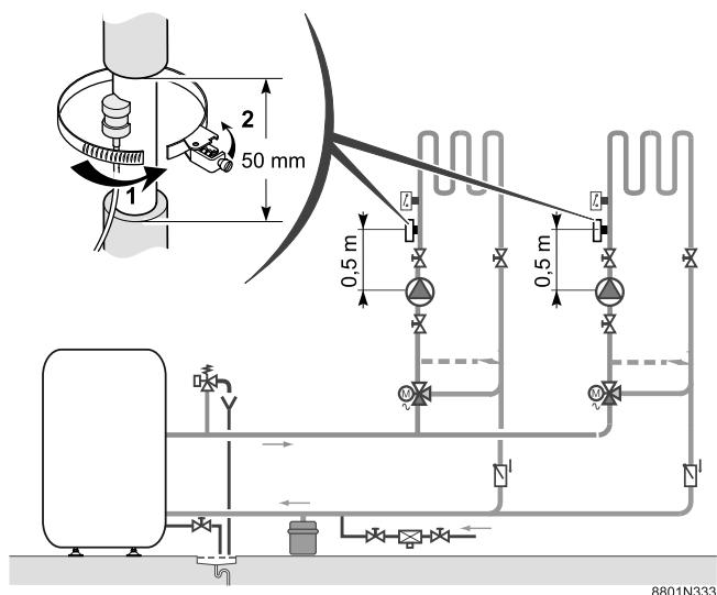
The flow sensor with connecting cable (length 2.5 m) and connector plug should be fitted to the outlet circuit pipe concerned and must be connected to the point provided in the control panel shown below.
